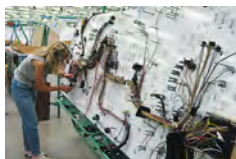
On-board Cable Testing
